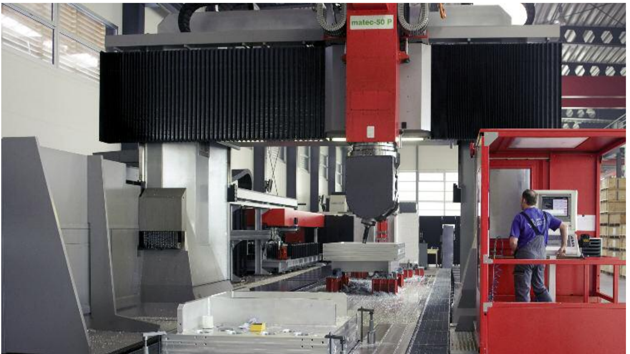
Klantspecifieke variant matec-50P met 2-assige CNC-motorspulfreeskop, meelopend bedieningsplatform, X = 16000 mm, Y = 5000 mm, Z = 1500 mm, W = 800 mm
